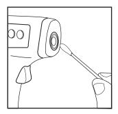
Clean the sensor periodically to ensure an accurate reading. Please use a cotton swab with 70% concentrated alcohol to clean the sensor. Allow the sensor to dry for at least 1 minute before the next measurement or use a tissue paper to dry it.
