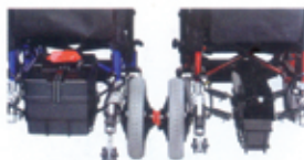
36AH BATTERY BOX 12793 17AH BATTERY BOX 12792
